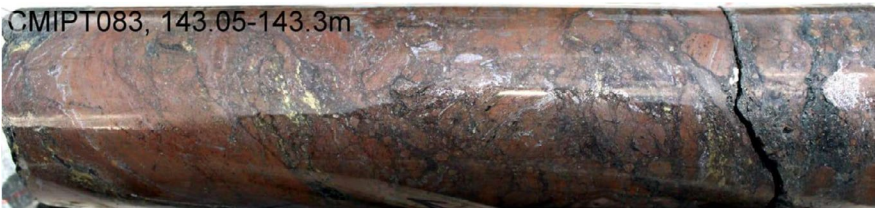
Figure 11: Second massive sulphide unit in drillhole CMIPT083: massive and brecciated massive sphalerite (red-brown) with lesser galena, with up to 3% chalcopyrite (yellow) present in places. There is inherent uncertainty in reporting visual results which may only be confirmed through laboratory analysis. Refer to Appendix 3 for JORC Table 1 information.
